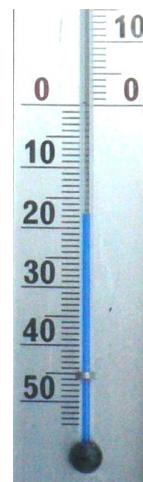
Fig. 1. Thermometer based on liquid thermal expansion.
