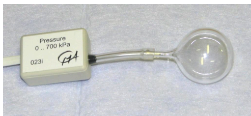
Fig. 4. Gas thermometer - glass bulb coupled with pressure sensor
