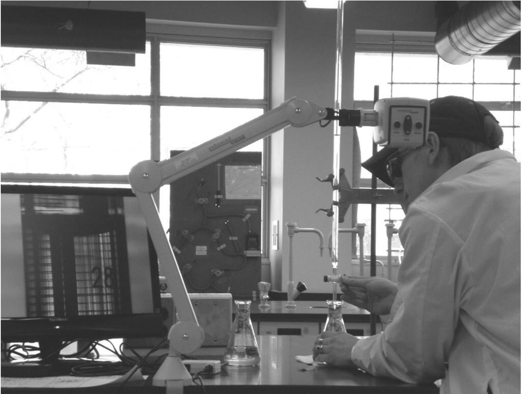
*Figure 1.* The apparatus being used in the distance view during a titration. The meniscus and the gradations of the burette are seen on the LCD screen at the left.
