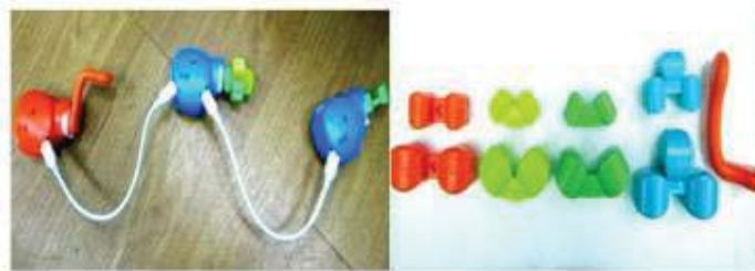
Figure 3: Actives (left) and passives (right) in Topobo system
