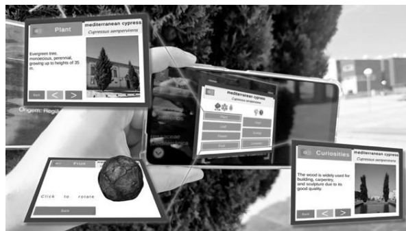
Figure 2. An example of a plant species AR Book content, triggered through 2D marker detection
