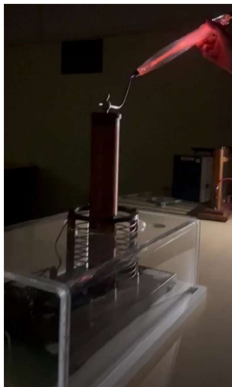
Figure 3. A Tesla coil lighting a Neon lamp at the Liceo “G. Berto”
