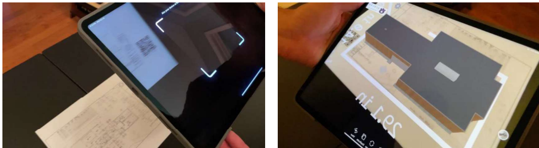
Figure 3. Scanning for AR Image Used by the Test Group (Scan Process on the Left and AR Image on the Right)
