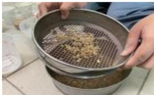
Figure 1: Sieve materials before weighting process
