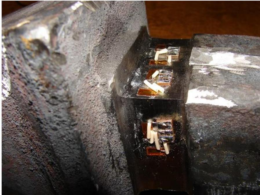
Figure. 8: Strain gauges bonded on the dynamometric tooth
