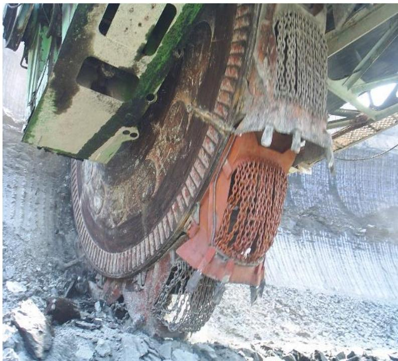
Figure. 2: Dynamometric bucket mounted onto RS1300 excavator type
