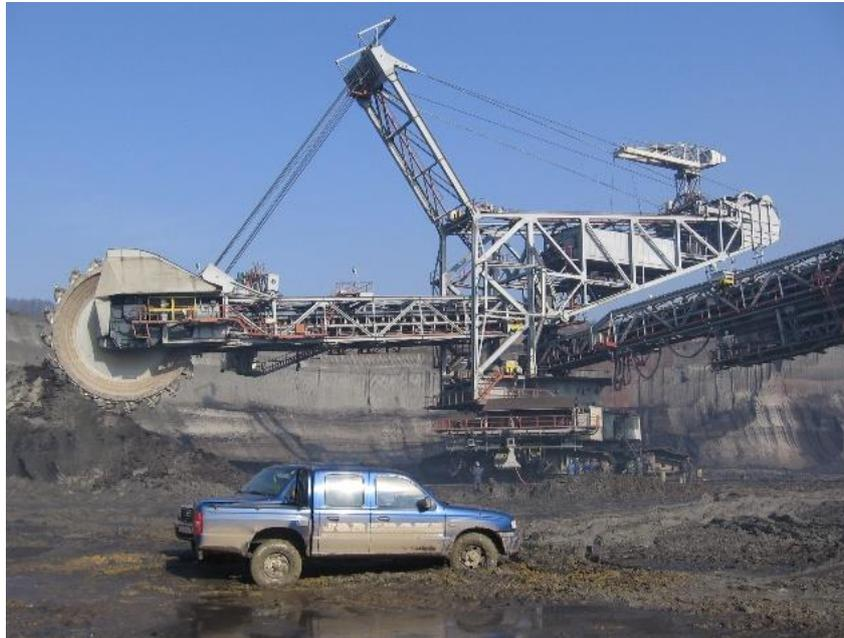
Figure.1 RS 1300 Excavator type in the mining field
