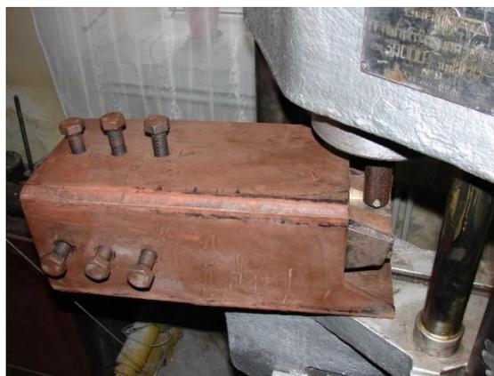
Figure. 13: Dynamometric tooth calibration in laboratory
