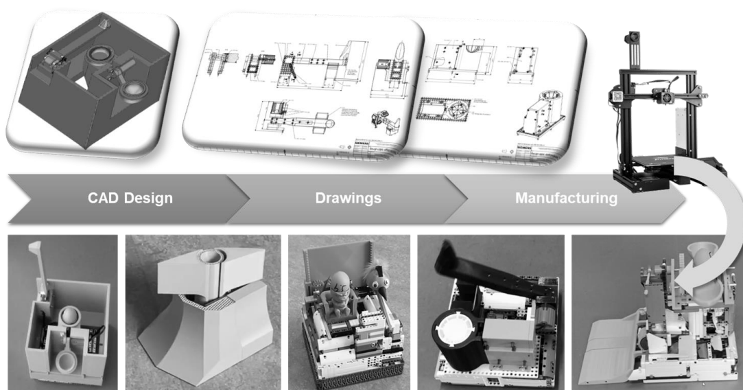
Figure 4. CAD designs and final 3D printed prototypes (phase 3 and 4).
