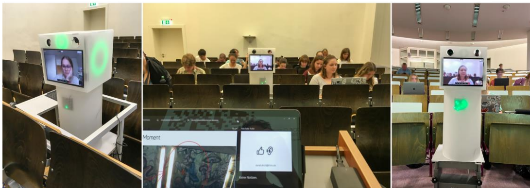
Figure 2. Functional prototype of the Fernstudent in the lecture hall during the field test.
