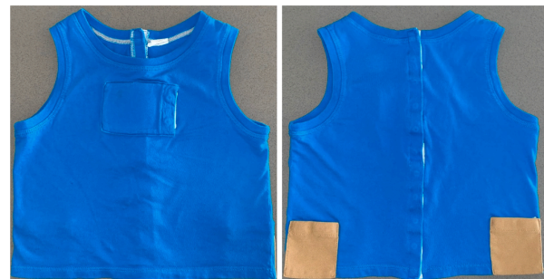
Fig. 1. Preschooler vest for wearable sensing technology. Note: 1A. Front of vest with pocket for LENA Digital Language Recorder. 1B. Back of vest with pockets for left and right Ubisense (location tracking) tags. Photo courtesy Catalina Cepero.
