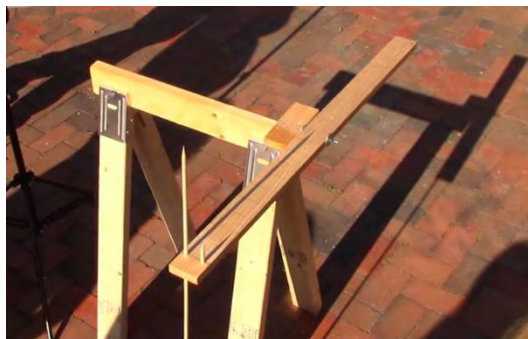
Figure 2. A SunRule consists of a ruled board (shadow plane) and rods that are orthogonal to the ruled board. By changing the angle of the shadow plane, one changes the length of the shadow of the shorter rod, which serves as the multiplicative unit. The height of the longer gnomon represents the multiplicand. The device works because rays from the sun are parallel.
