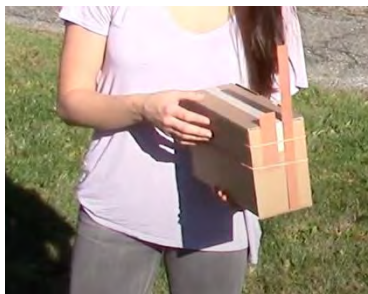
Figure 7. Sara inclines the device less toward the sun, which decreases the sun’s apparent altitude and causes the shadows of the gnomons to lengthen.
