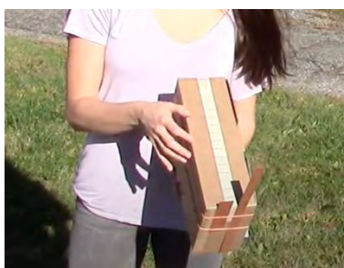
Figure 6. Sara inclines the device more toward the sun, which increases the sun’s apparent altitude and causes the shadows of the gnomons to shorten.
