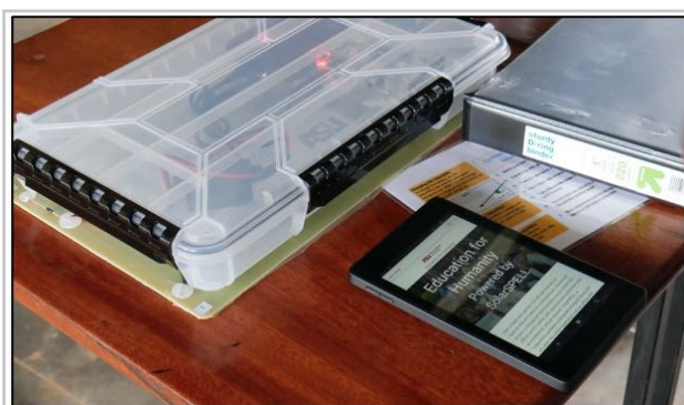
© ASU Education for Humanity The SolarSPELL device is housed in a ruggedized plastic container.
