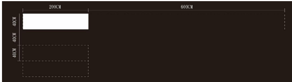
Figure 2. Production Method of the Crosswalk
