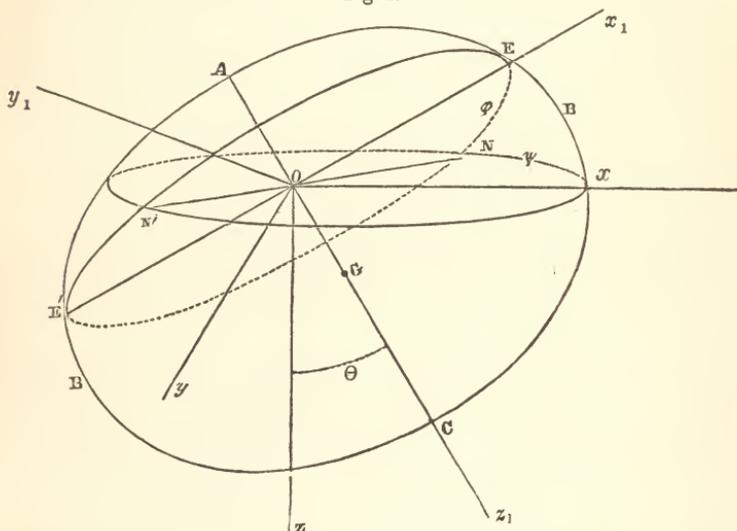
For the purpose of determining the axes  $Ox_1, Oy_1$  and  $Oz_1$ , with reference to the (fixed in space) axes  $Ox, Oy, Oz$ , three auxiliary angles are used.
