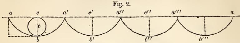
horizontal plane, and whose sagittae  $cb, c'b', \&c.$ , are to the amplitudes  $aa', a'a'', \&c.$ , as  $\frac{\sin \alpha}{2\beta^2} : \frac{\pi}{2\beta^2} :: \sin \alpha : \pi$ . If the initial elevation  $\alpha$  is  $90^\circ$ , this ratio is *as the diameter to the circumference of the circle*: a property which indicates the *cycloid*.
