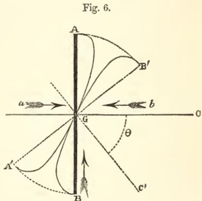
The *centrifugal* forces due to the deflections of the vertical motions are normal to the concavities of these curves; hence, on the side of the axis towards the eye, they are to the left, and on
