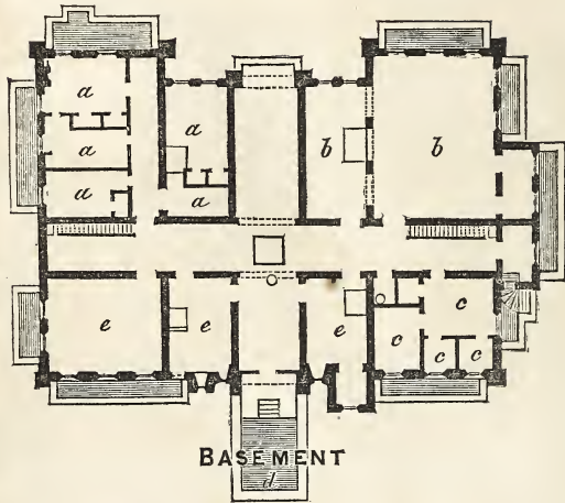
Fig. 5. BASEMENT. a. a. a. a. Residence for a Professor. b. b. Gymnasium. c. c. c. Janitor's apartment. e. e. e. Store-rooms and Work-shop. d. Coal vault.
