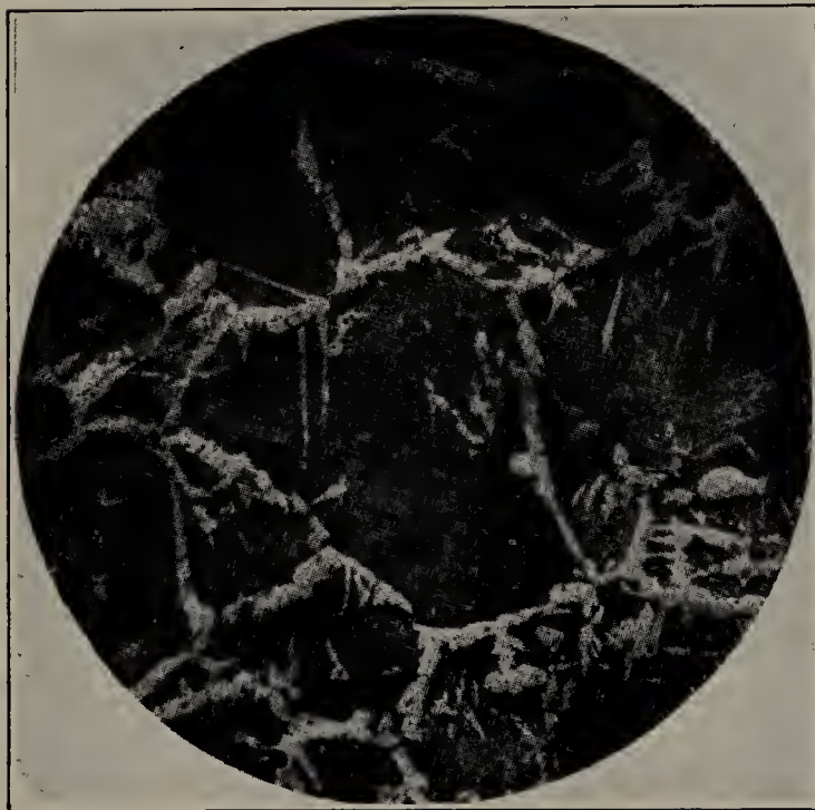
FIG. 7.—STEEL RAIL, MAGNIFIED 100 DIAMETERS. MADE OF GOOD STEEL, BUT ROLLING FINISHED AT TOO HIGH A TEMPERATURE
