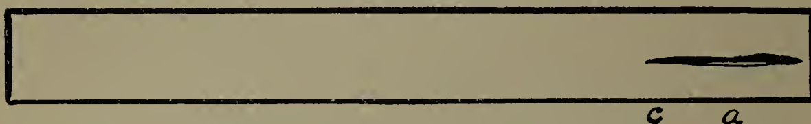
FIG. 4.—DIAGRAM OF THE PIPE IN A "BLOOM," A PARTIALLY ROLLED STEEL INGOT
