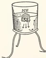
Ice causing downward and upward currents.
