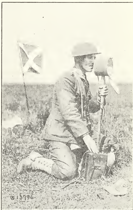
FIG. 174. A member of the Signal Corps using a sunlight flash signaling apparatus. (Photograph, Committee on Public Information.)
