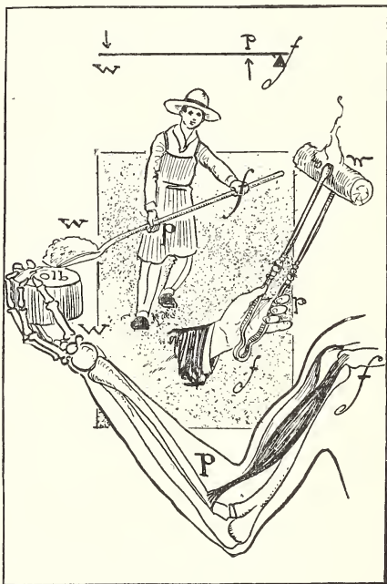
FIG. 166. Levers of the third type. Explain each case.
