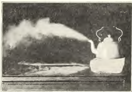
FIG. 12. A kettle of liquid air boiling on a block of ice. (Courtesy, Professor Louis Derr.)
