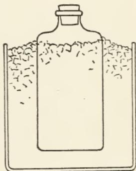
What causes pipes to burst in freezing weather?
