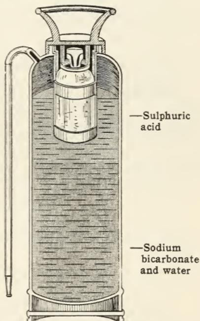
The small bottle contains sulphuric acid and the larger vessel contains sodium bicarbonate and water. Explain how this fire extinguisher works.
