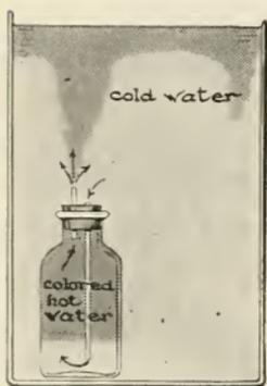
What causes the warm colored water from the small bottle to rise to the surface of the cold water in the larger vessel?
