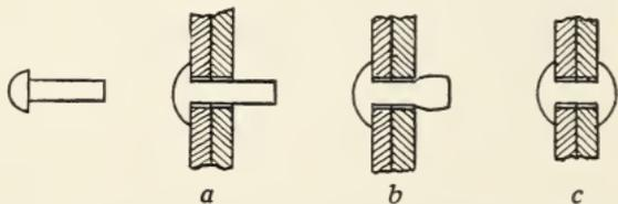
Why are rivets heated white hot before they are inserted into steel plates?
