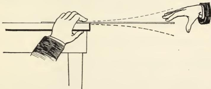
A vibrating stick. How can the pitch of sound produced by the vibrating stick be varied? How may the intensity of the sound be varied?
