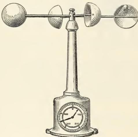
The anemometer. From two Greek words meaning "measure of wind." Why are the vanes cup-shaped?
