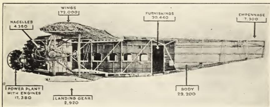
Thousands of pieces of metals and wood are used in the construction of a plane.
