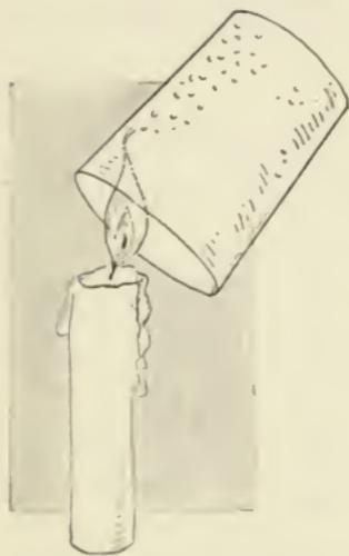
**Demonstration.** To show that oxygen and hydrogen combine to form water. Light a wax candle and carefully hold a cold glass, mouth down, over the flame. After a short time the oxygen in the glass is used up and the candle is extinguished. What is found on the inner surface of the glass? Where did it come from?
