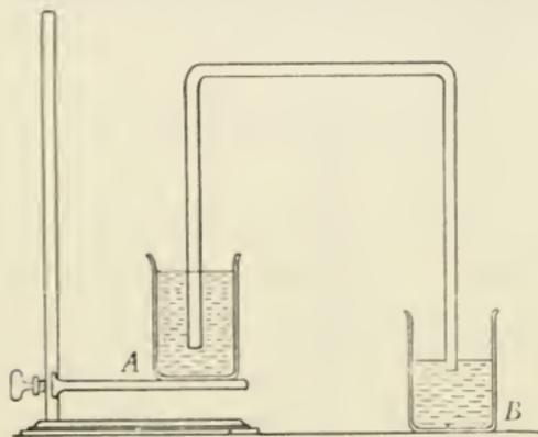
**The siphon.** Normal pressure of air may be used in transferring liquids from one vessel to another vessel at a lower level. The air pressing down on the
