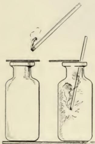
**Demonstration.** To show that oxygen will support burning. Obtain some sodium peroxide and drop a very small portion of it into a glass jar with a narrow neck containing a delivering tube. Add a little water. Collect a bottle of the gas given off. Insert a glowing splinter into the jar of gas. Note how the lighted end of the stick behaves. Blow out the
