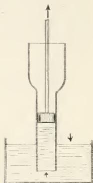
In a lift pump, the chimney is known as the *cylinder*, the rubber stopper is the *piston*, and the basin of water is the *well*.
