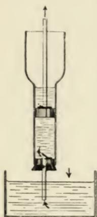
Let us now see if we can understand the action of the lift pump, shown in the diagram. As the handle is moved down, it lifts the piston upward in the cylinder. This reduces the air pressure in the lower part of the cylinder, and the water rushes up from the well, opening the valve, *B*, at the top of the shaft. At the same time, the piston valve, *A*, closes. The cylinder is now partly filled with water, be-
