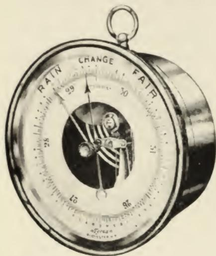
An aneroid barometer. Air pressing against a diaphragm to which is attached a spindle causes the spindle to move. The indicator attached to the spindle registers the amount of this motion on a dial. When the air pressure is increasing, the indicator moves toward the right; when the air pressure is decreasing, the indicator moves to the left. How does the indicator move when the barometer is carried in an airplane to a high altitude? To a lower altitude?
