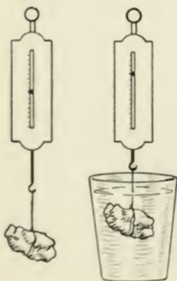
stone by suspending it from the hook of a spring scale, as shown in the illustration. Record the weight in your notebook. Still keeping the stone suspended from the scale, lower it slowly into a vessel of water until it is entirely submerged. Be careful not to let it touch the sides or bottom of the vessel. Read the scale now. Does the stone weigh more or less in water than it does in air?
