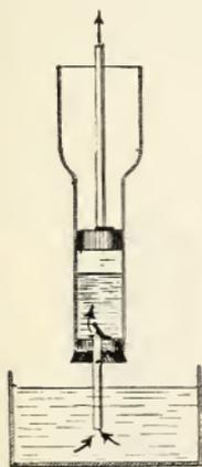
With a small piece of leather and a thumb tack make a little cover for the upper end of the tube. Such a cover is like a little trap-door and is known as a *valve*. With both stoppers in position, hold the chimney so that the lower end of the glass tube is immersed in the basin. Draw the upper stopper sharply upward as before. Does the water rise in the tube? Why? Does it pass through the valve and rise in the lamp chimney? Now replace the upper stopper with one the same size but
