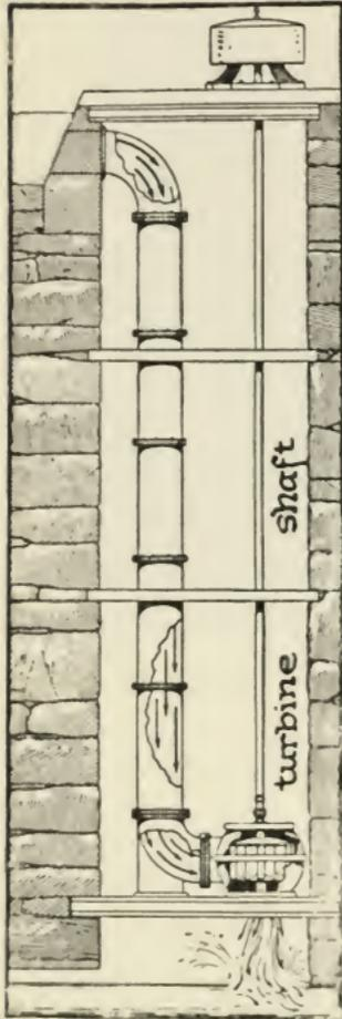
Water turbines supply power. Why are the turbines located near the bottom of the water fall?
