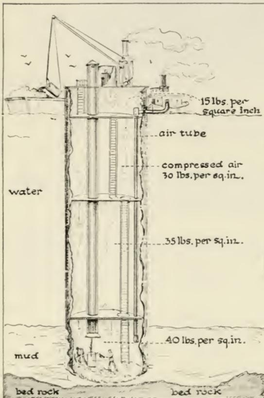
Cross section of a caisson. Why does the air pressure differ in the various chambers? How are the men able to stand the pressure of 40 pounds of air per square inch?
