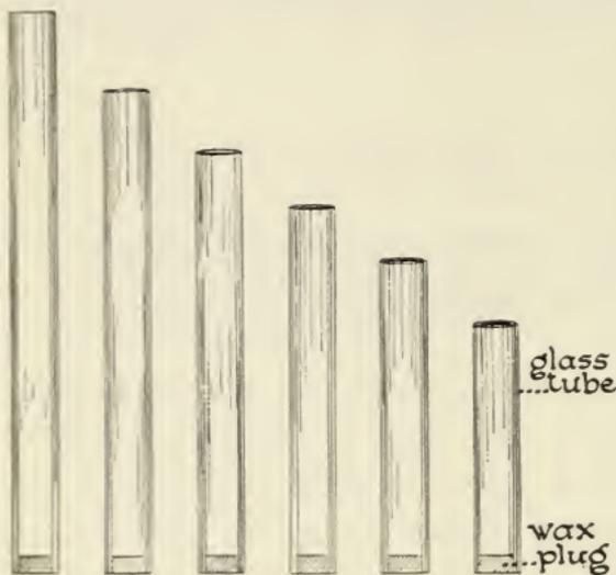
tube, blow sharply. Are the resulting sounds equal in pitch? How does the length of the tube affect the pitch?
