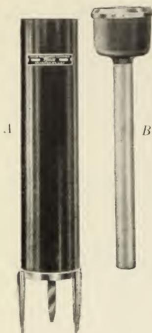
A rain gauge. A is a container into which the rain gauge, B, fits. On which part of the instrument would you look for the scale which indicates the amount of rainfall?
