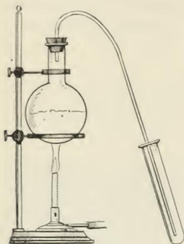
the tube into an empty test tube. Heat the flask over a Bunsen burner. What happens to the water? When the water starts to boil, what appears in the test tube? Where did they come from? What is the color of the water in the test tube? Does it taste sweet? This process of purifying water is known as *distillation*. What effect does distillation have on water?
