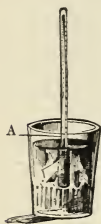
FIG. 246.—The temperature of melting ice is called the temperature of zero ( 0^{\circ} ).
