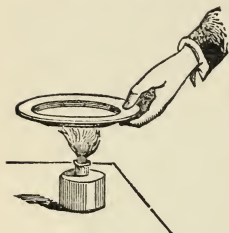
FIG. 261.—There are drops of water formed. This water is due to the combination of the hydrogen of the alcohol with the oxygen of the air.
