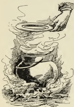
FIG. 235.—Steam becomes a liquid on coming in contact with a cold plate (liquid state).
