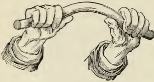
FIG. 231.—The lead pipe can be twisted in all directions. Lead is flexible.
