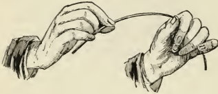
FIG. 232.—The steel needle straightens when released. It is elastic.
