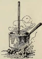
FIG. 245.—The temperature of boiling water is called the temperature of 100 degrees.
