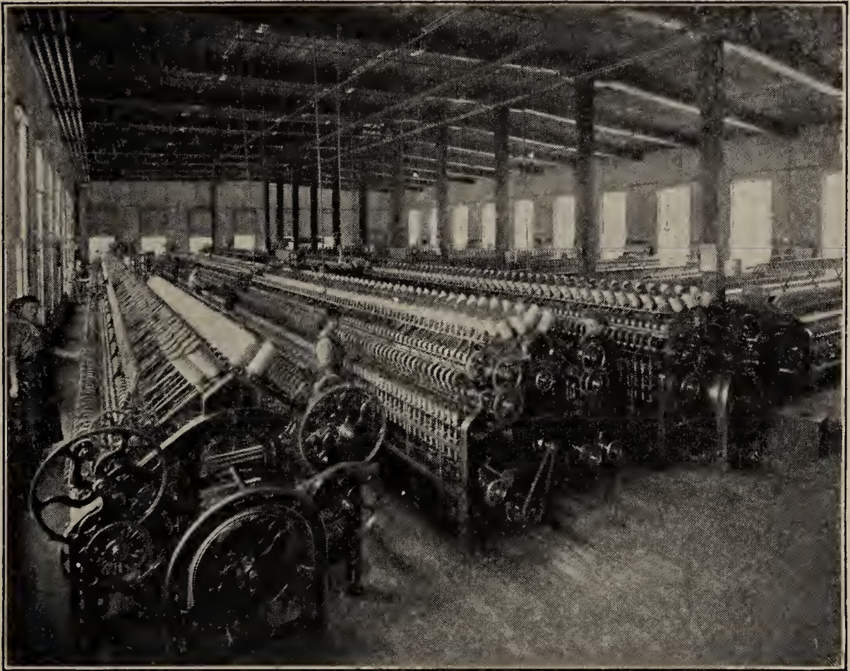
FIG. 56. — One person can supervise many machines in the spinning room of a cotton factory.
