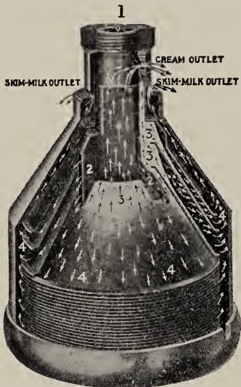
FIG. 284.—Showing the construction and operation of the cream separator.
