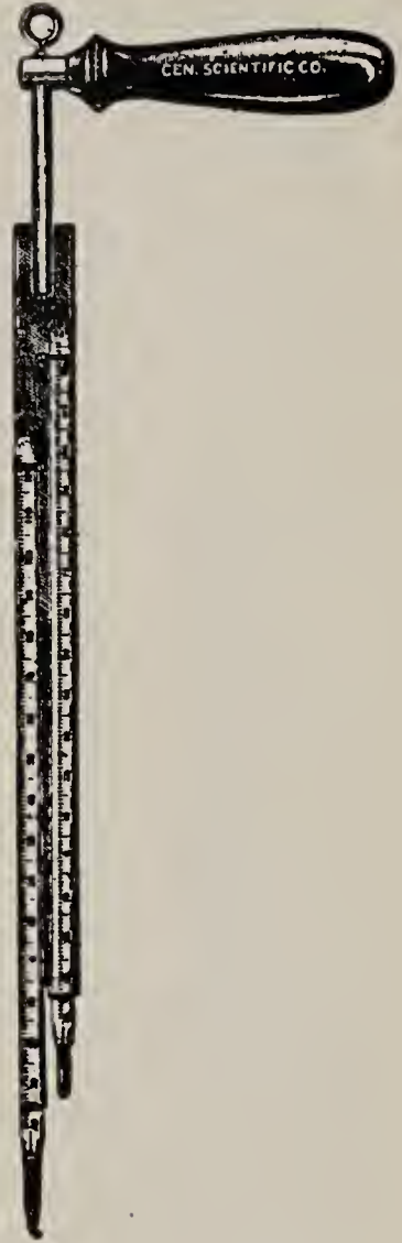
FIG. 119.—The sling psychrometer. The lower bulb is covered with muslin and is moistened before an observation. The thermometers are then whirled about the hand, and read every half minute or so till the wet thermometer ceases to fall lower.
