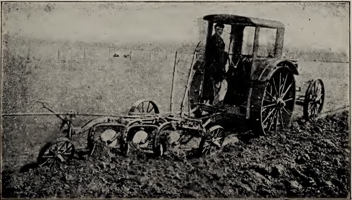
FIG. 290.—A farm gasoline tractor pulling a three-bottom plow and doing the work of 6 or 8 horses or of 50 men.
