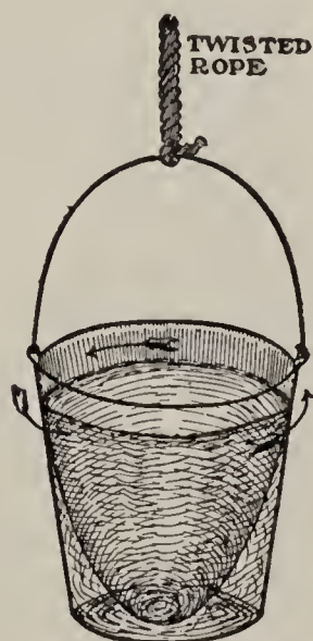
X-ray view. Centrifugal force holds water against side of pail.
