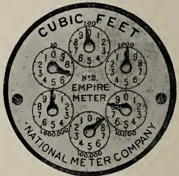
FIG. 255.—The dial register. It reads 987,997 cu. ft.
