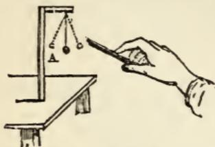
FIG. 62.—The little ball of elder pith is repelled as soon as it touches the wax A that has been rubbed.
