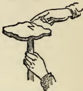
FIG. 65.—I place my finger near it, and I obtain little sparks, and a slight crackling noise.
