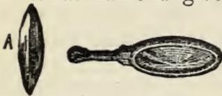
FIG. 35.—Double *convex* lens (rounded on both sides).
