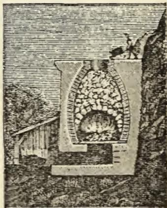
FIG. 90.—Lime-kiln. When calcareous stones are subjected to a very high temperature they are transformed into lime.
