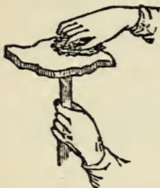
FIG. 64.—I rub the resin with a piece of woollen cloth.
