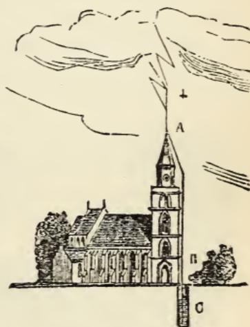
FIG. 75.—If a thunderbolt falls, it follows in preference the rod AE and is lost in the earth C.
