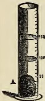
FIG. 103.—The level of the water, which was at 100, rises to 160: the difference indicates the volume of the lead A.
