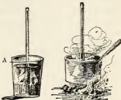
FIG. 17. — Thermometer plunged into *melting ice*. Temperature, 32°.
