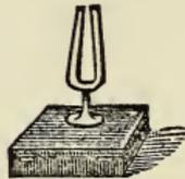
FIG. 57.—If I place the tuning-fork on a wooden box (*sounding-board*) the sound becomes stronger.
