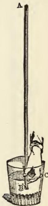
FIG. 113. — The tube closed at A, open at B, remains full of water, and does not empty itself in the glass. It would be the same for a tube that was 11 yards high.
