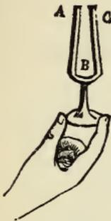
FIG. 56.—Tuning-fork. A, B, C, branch of steel which when set vibrating gives the A that has 806 vibrations in a second.
