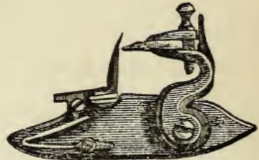
FIG. 92.—Lock of a gun. It is the spark that inflames the powder.
