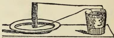
FIG. 81.—The water is decomposed into gas (oxygen and hydrogen) by the electric current (chemical effect).
