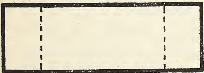
(a) BEND AT DOTS WITH RULER TO CREASE IT
