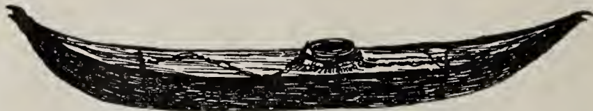
Seal skin boat (bidahkah) of the Aleutian Islander, used by the natives in capturing the sea otter and seal. Drawn by Wm. A. Davis, Principal U. S. Public Schools, Unalaska, Alaska.
