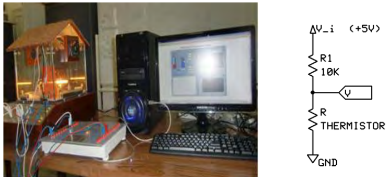
Figure 3. Temperature regulation room and the connection of NTC Sensor
