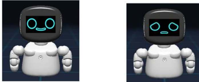
(a) Facial expression for correct answer (b) Facial expression for Incorrect answer
