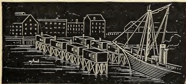
Blackboard Drawing of a floating Dry-Dock. Water let into dock, which sinks to receive vessel.
