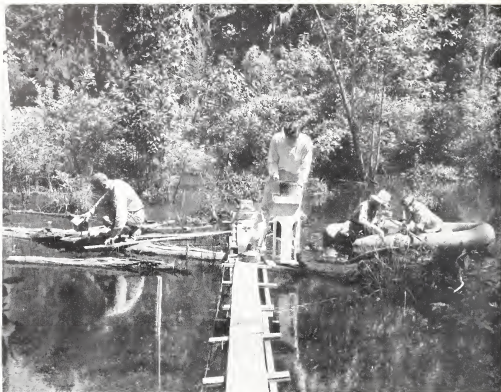
An observation station showing activities in studying pond: At the left, taking a reading of wind velocity on the surface of the water by means of a Baumanvenometer; center, taking readings of rainfall on rain gauge at left, dipping for mosquito larvae from a portable rubber boat.
