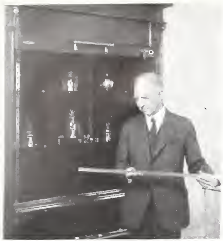
Interior view of the vault at the National Bureau of Standards in which the standards of length and mass of the United States are kept. Dr. Lyman J. Briggs, Director of the Bureau is shown holding the national standard of length, Meter No. 27.
