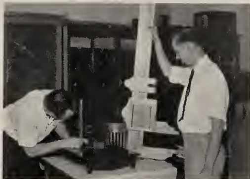
Future graduates of a trade course getting training in use of Vernier height-gage and Vernier calipers.
