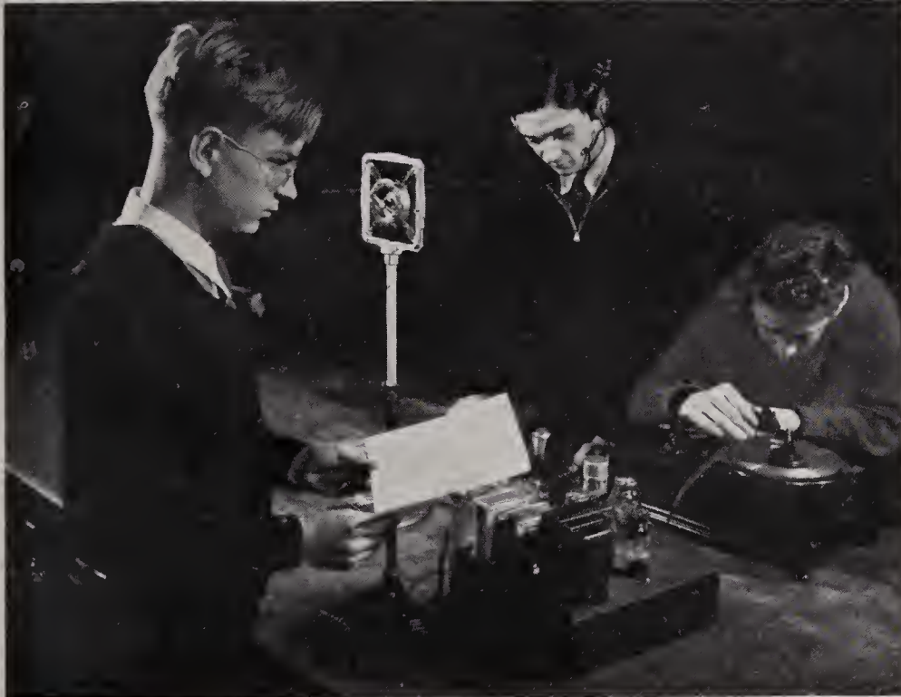
In the picture above is shown the recording of a voice on a disk. The microphone picks up the sound waves of the speaker's voice and converts them into electrical impulses. These students are intrigued by their experimentation in the physics laboratory.
