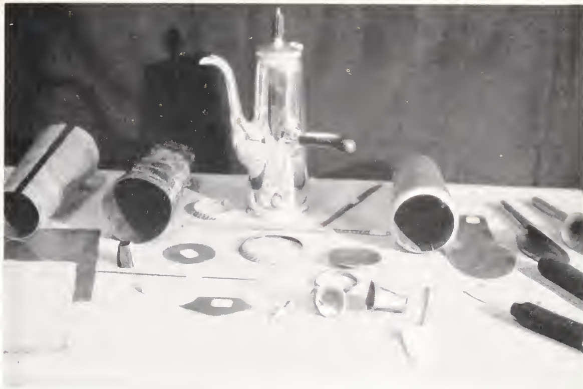
This illustration shows various parts of a silver coffee pot made by students in silversmithing course at Meriden, Conn., Trade School and the final product fabricated from these parts. This material is now on exhibit in the Office of Education section of the Museum. It is in one of the several cases devoted to various fields of education
