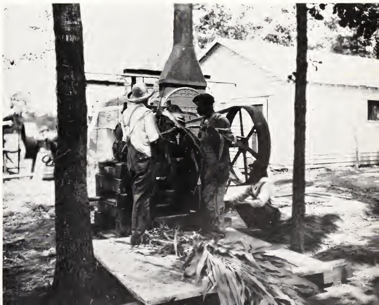
Crushing juice from sorghum cane in the syrup mill owned by the community cooperative association established and operated by farmers attending classes in the Ellen Woodside School, Pelzer, S. C.
