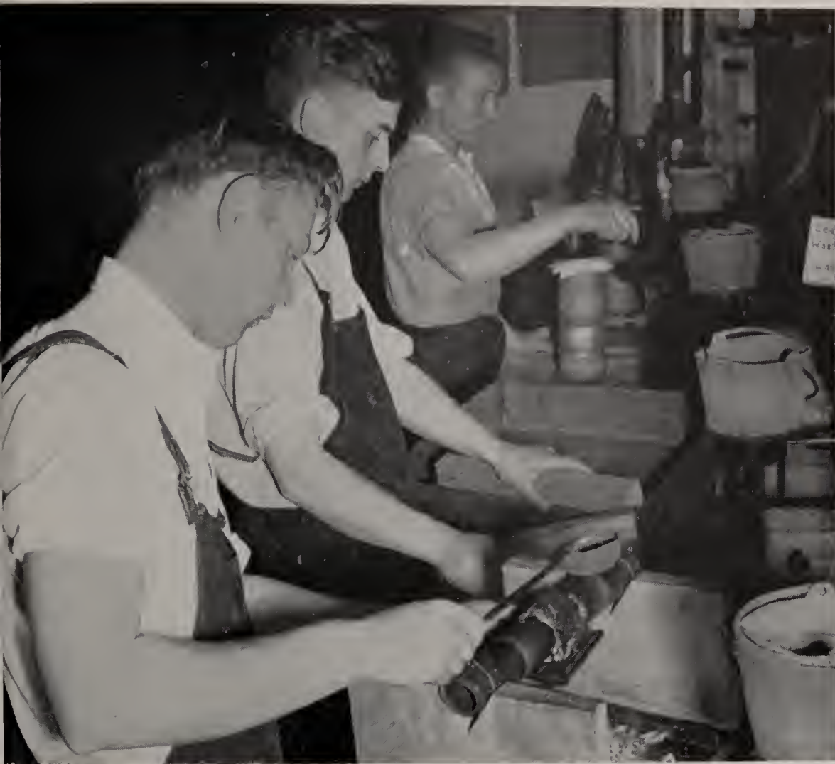
Lead wiping is one of the types of work which may have to be taught the plumber apprentice in the classroom when the employer is unable to give this instruction.
