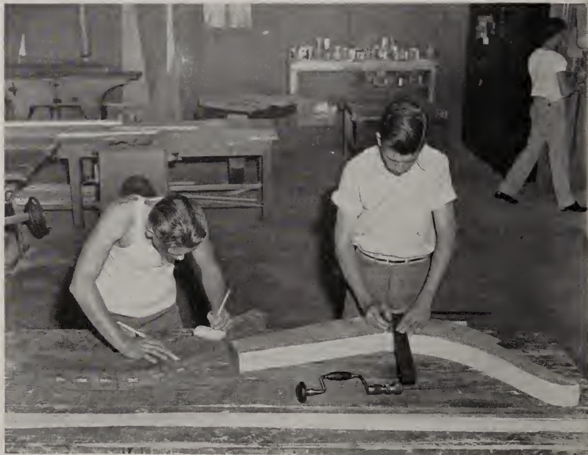
Courtesy, Miami Technical High School. Future boat builders in Miami Technical High School, laying out members of boat structure.
