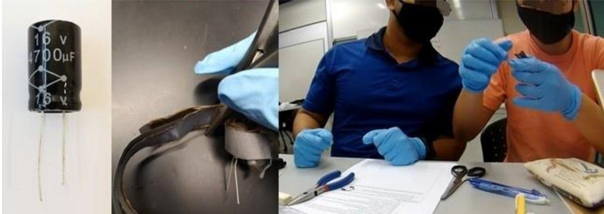
Figure 2 The dissection of aluminium electrolytic capacitor.
