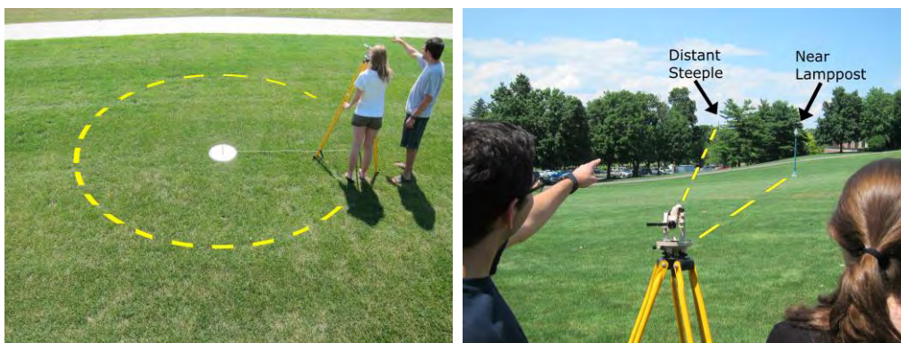
Figure 1. Setup for terrestrial parallax measurements. Students lay out a circular "orbit" from which to make measurements (left). Using a surveyor's transit, they measure the angular separation between a nearby object and an object in the distant background (right).
