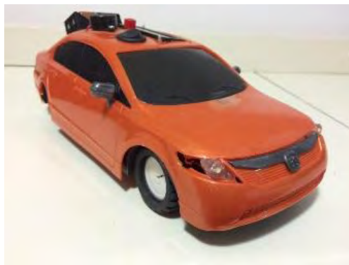
Figure 2. Automated toy car as a robotics learning platform.
