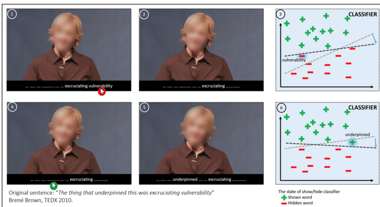
Figure 1. Learner feedback on the caption to hide a word (top) and to show a masked word (bottom) by clicking on it. The classifier’s labels and the decision boundary (dashed line) change according to the learner feedback
