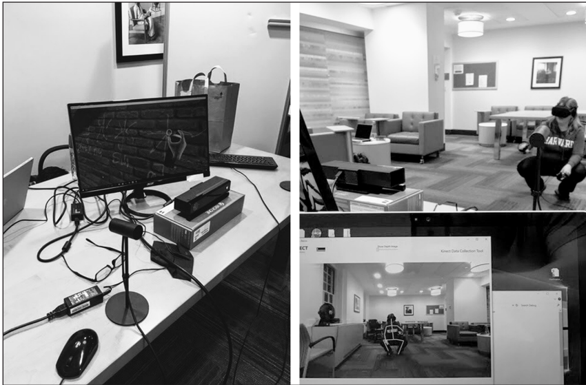
Figure 1. Set-up of the experimental VR condition ( Left : The Oculus Rift sensor in the foreground and the KinectTM sensor in front of the monitor; Right : A participant (background) squatting down while using the Oculus Rift and the KinectTM software (foreground) recording her movement on a laptop)
