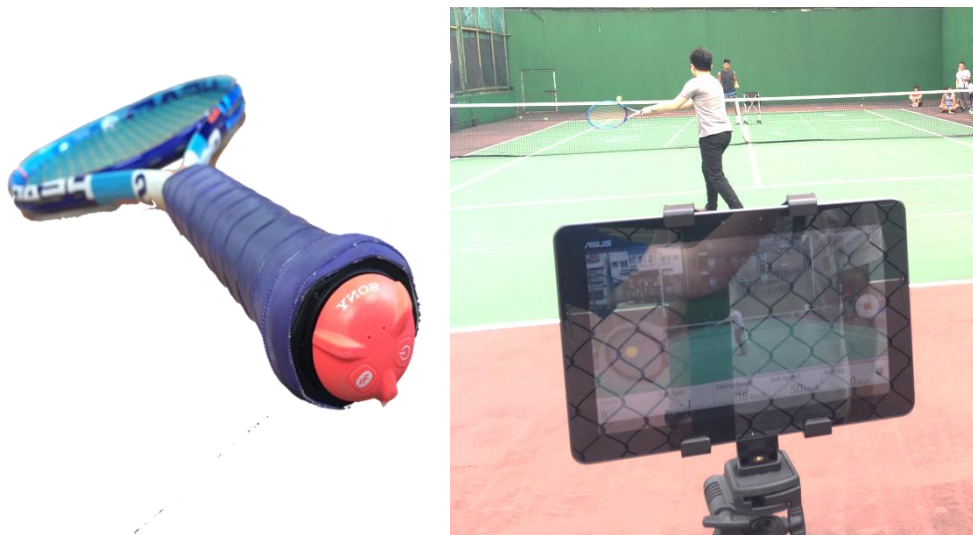
Figure 1. (a) A Racket attached with a Sensor; (b) A Tablet, Synced with the Sensor, is filming a Student's Practice
