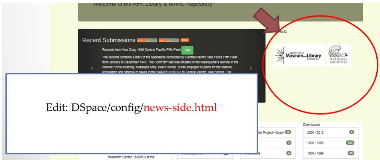
Figure 5. The right-side news bar can be changed by editing the news-side.html file in coded html text.
