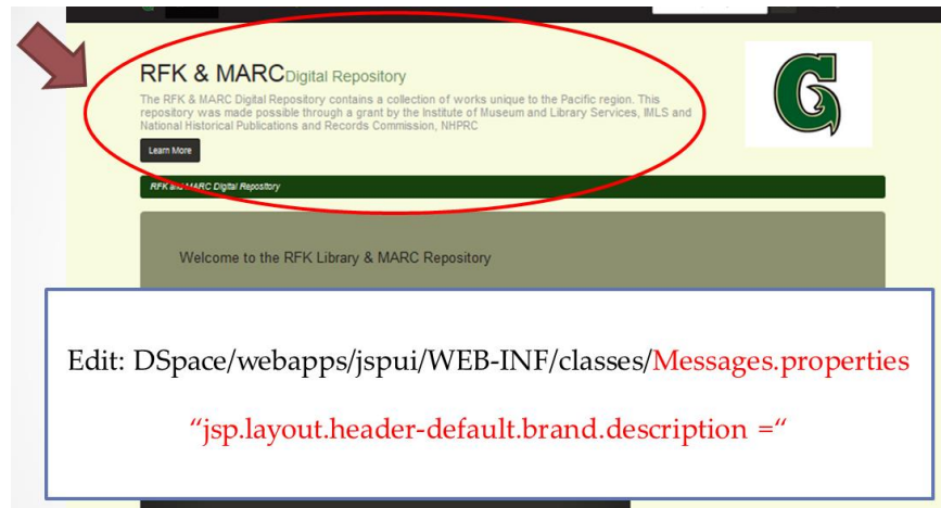
Figure 2. The header message can be edited by changing the jsp.layout.header-default.brand.description value in the message.properties file.
