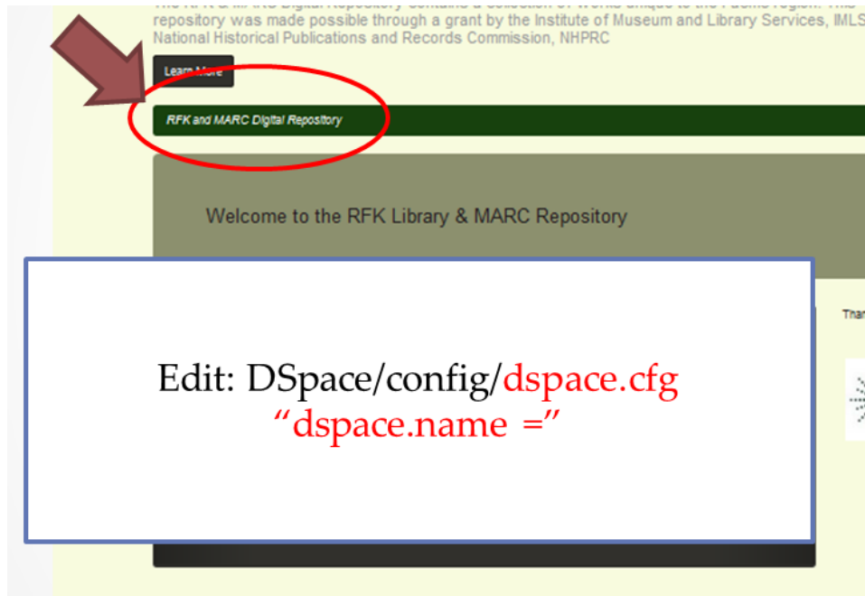
Figure 3. The repository title can be edited by changing the dspace.name value in the dspace.cfg file.
