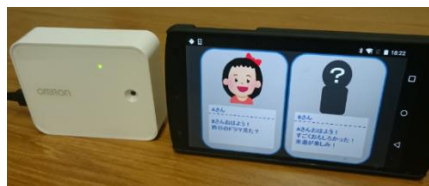
Figure 1. A face sensing sensor HVC-C (left) and a question mode screen on a smart-phone (right)
