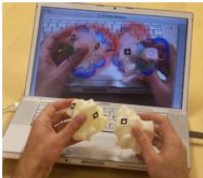
Figure 7. Augmented reality tangible molecular interface showing manipulation of two 3D printed physical models of subunits of the enzyme Cu-Zn superoxide dismutase, augmented on the computer screen with the electrostatic potential fields that are computed for the two subunits.
