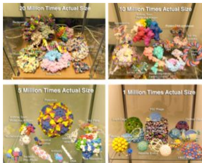
Figure 2. 3D printed molecular models at various scales. Full color models are made with the powder-based Z Corp printer. Monochrome models are made with the FDM Stratasys printer
