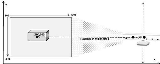
Figure 1. Depth Data Processing [2] of Kinect Sensor
