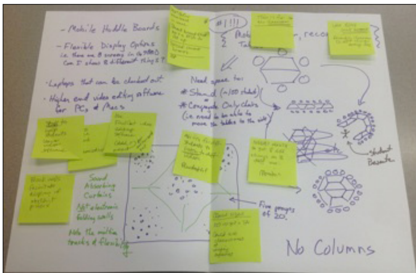
Fig. 5: Example of a faculty drawing showing required flexibility in space (movable furniture, soundproof curtains to divide the room, and related features)
