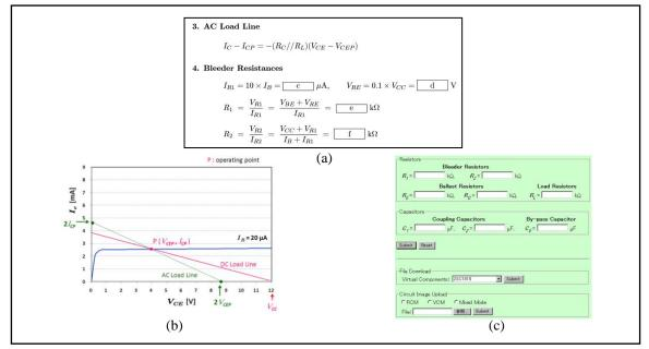
Figure 4. (a) Operating point and load lines that are indicated on  $V_{CE}$ - $I_C$  characteristics, (b) manual to calculate the circuit parameters, and (c) input forms to submit the information of the designed circuit.
