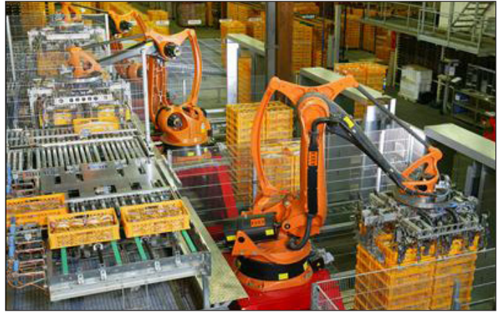
A factory robot puts bread onto pallets. Image © 2011 by KUKA Robotics Corporation. Used with permission.
