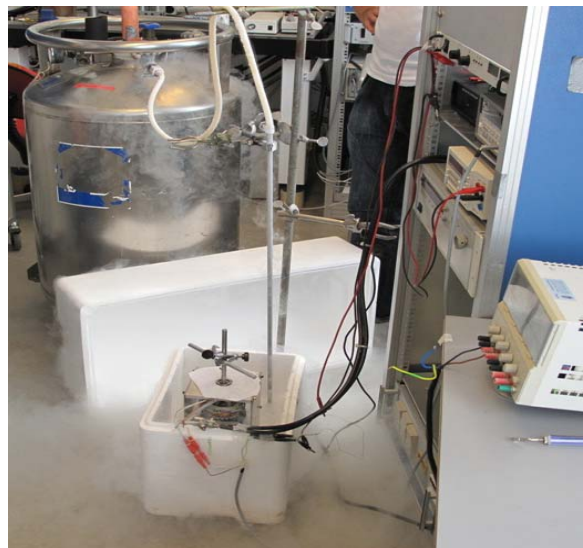
Figure 5. The HTS machine prototype setup after cool-down and during testing.
