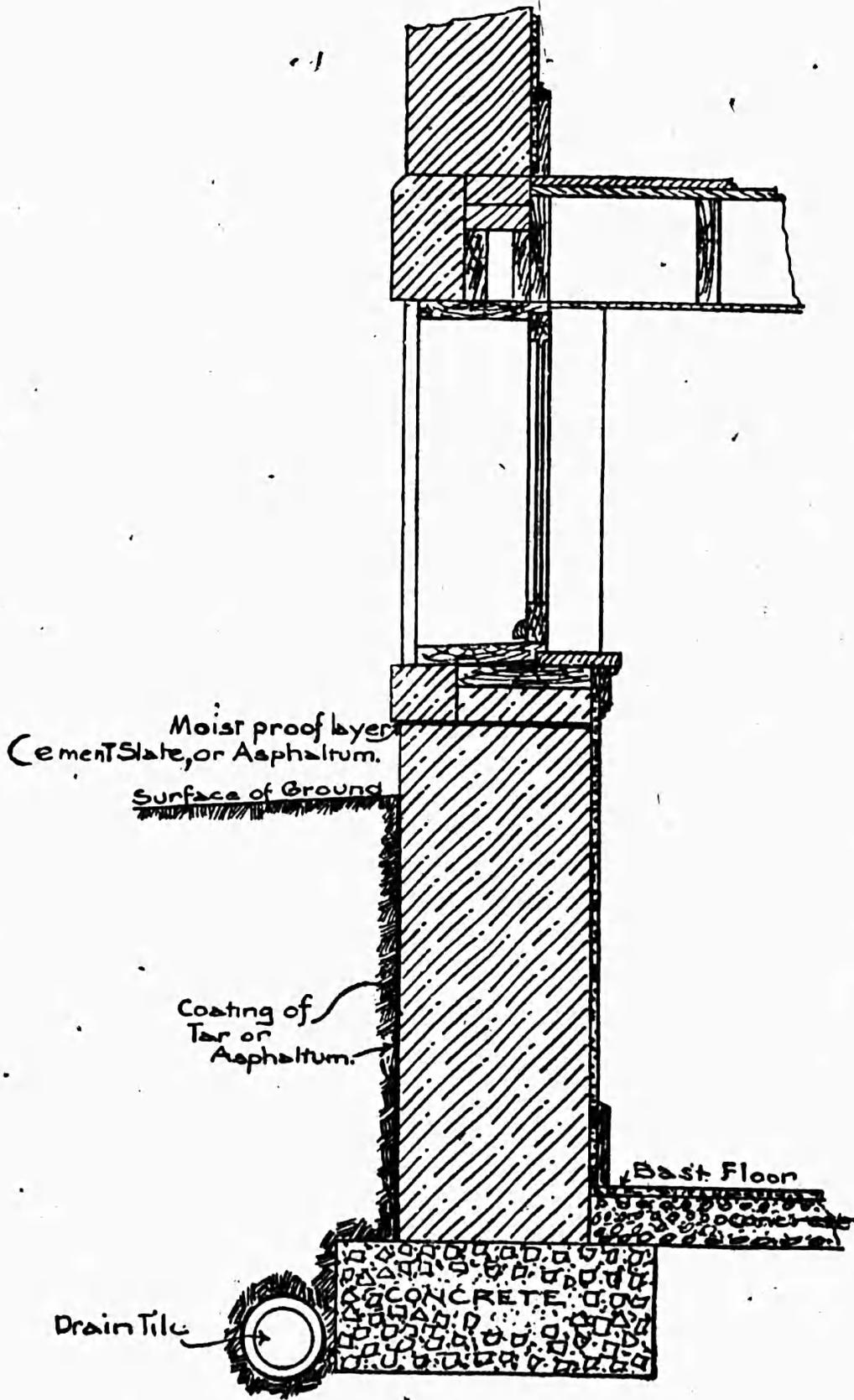
FIG. 1.—Section of foundation.
