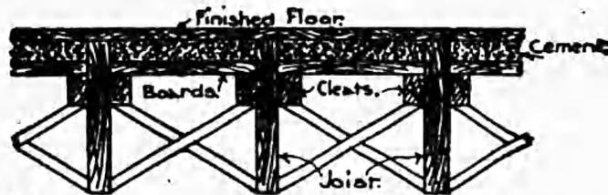
FIG. 4.—Floor with wooden joists and a thin layer of cement.
