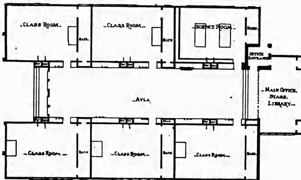
FIG. 7.—Plan for a village high school, so arranged that the hall may serve as an assembly room, with the main office as the stage.
