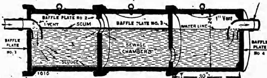
FIG. 5.—Septic tank made of glazed sewer tiles.
