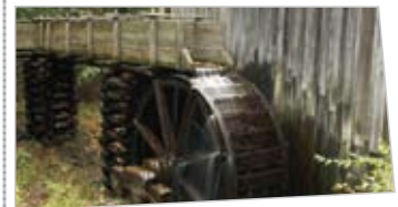
Pipes are often used to bring water from a river or stream to the top of an overshot wheel.
